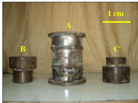
Fig. 2: Compression Chamber Assembly. A-Cylinder, B-Lower lid, C-Upper lid.
