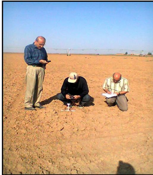
Fig. 3: Soil ECa in-situ measurements
