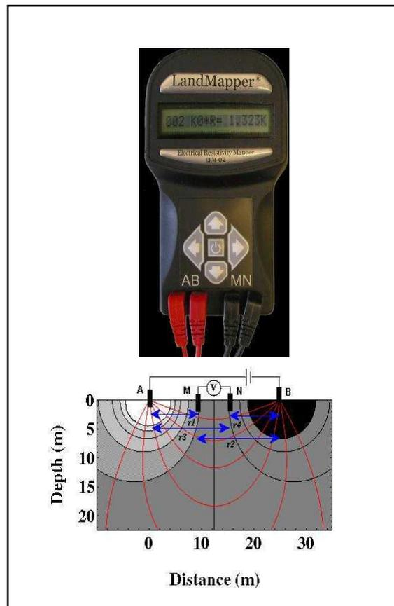
Fig. 4: Schema of current distribution in the soil by the LandMapper ERM-02 four-electrode probe(from [http:// Landviser.net/web\\_send/10](http://Landviser.net/web_send/10), 2013).
